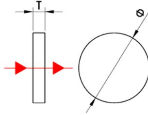
Zinc Selenide has wide transmission band, along with its low absorption in the red portion of the visible spectrum, Zinc Selenide is ideal for 10.6 $\mu$ m CO<sub>2</sub> laser system.
