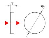
N-BK7(Chinese Equivalent H-K9L), a relatively hard galss, does not scratch easily and can be handled without special precautions.N-BK7 performs well in chemical tests such that special treatment during polishing is not necessary. The bubble and inclusion content of N-BK7 is less than 0.029mm2 per 100 cm3.N-BK7 has excellent transmittance as low as 350nm.
